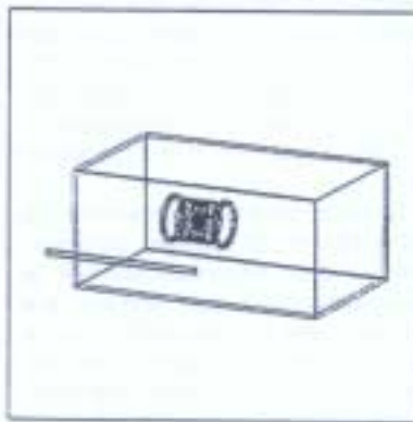
Figure 2. View of the Magnet Coils and the Surrounding Passive, Ferromagnetic Shield.
